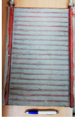
Figure 3. Tube–fin aluminum heat exchanger filled with activated carbon for a small-scale adsorption refrigerator, employing ethanol as the refrigerant [31].
